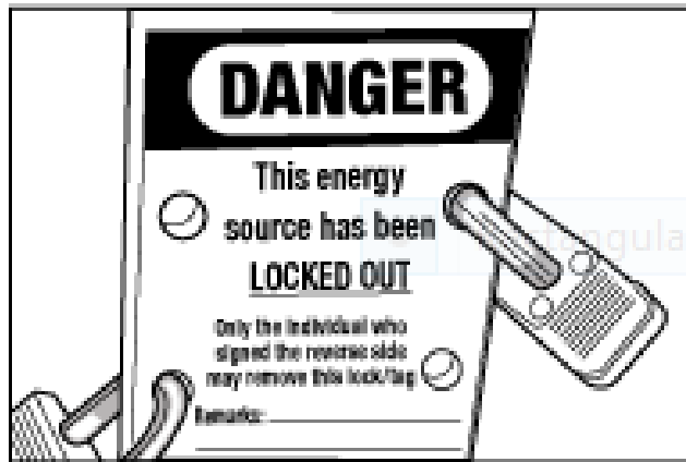
Figure 12 Example of multiple locks on a lockout tag
