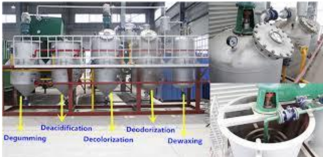
Figure 5 Edible oil refining equipment's
